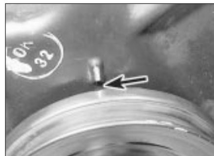
7.7 Ignition timing marks (arrowed) in alignment
