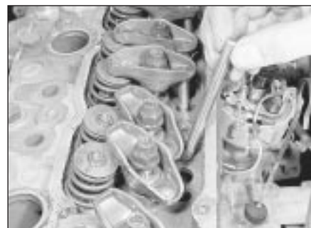
8.17 Removing the pushrods
