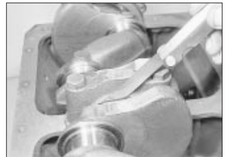
20.18 Checking the crankshaft endfloat
